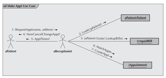
**FIGURE 7-10** Communication Diagram for a Scenario of the Make Old Patient Appt Use Case (Figure 6-10)
