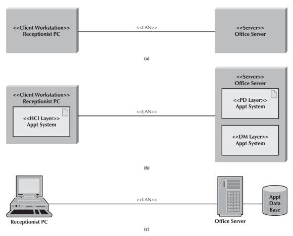
FIGURE 11-9 Three Versions of Appointment System Deployment Diagram
