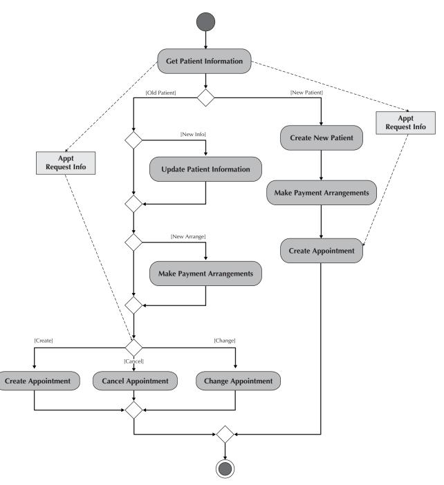
FIGURE 4-8 Activity Diagram for the Manage Appointments Use Case
