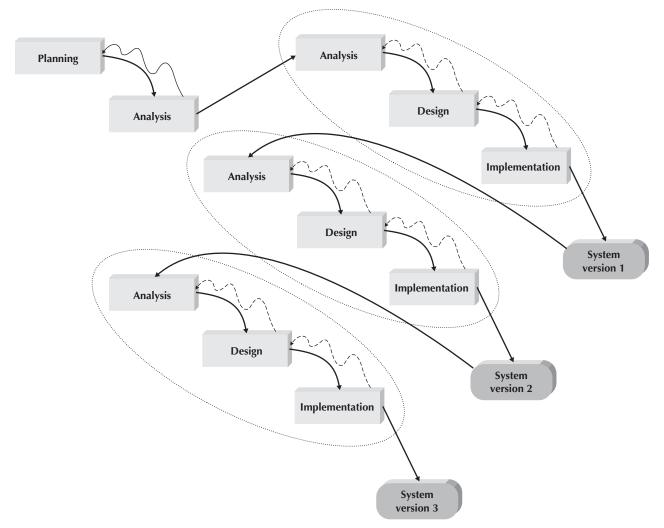
FIGURE 1-4 A Phased Development-Based Methodology
