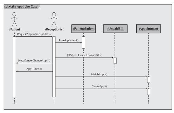
FIGURE 6-1 Example Sequence Diagram
