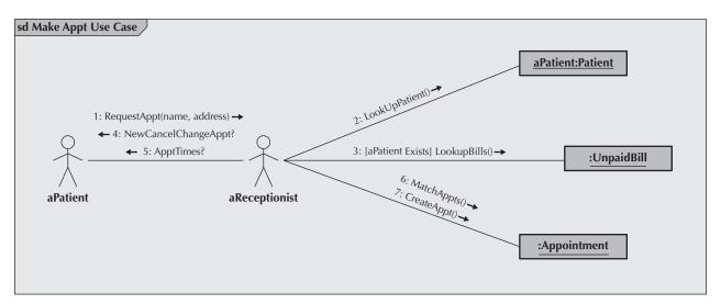
FIGURE 6-10 Sample Communication Diagram
