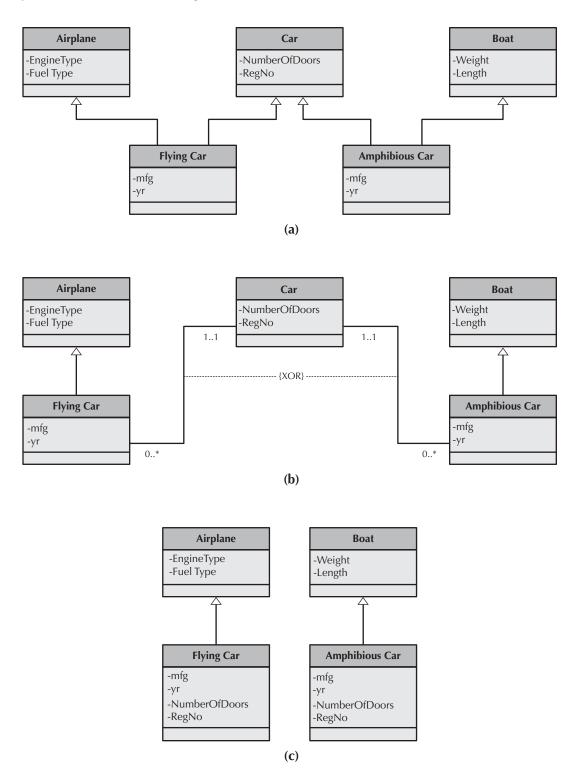
FIGURE 8-16 Factoring Out Multiple-Inheritance Effect for a Single-Inheritance Language
