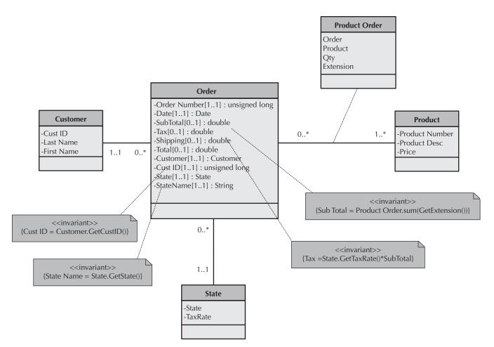
FIGURE 8-20 Invariants on a Class Diagram
