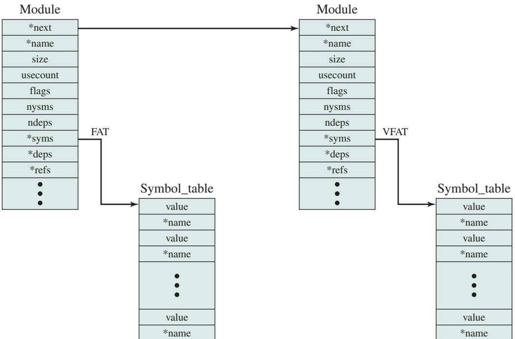
Figure 2.19 Example List of Linux Kernel Modules
