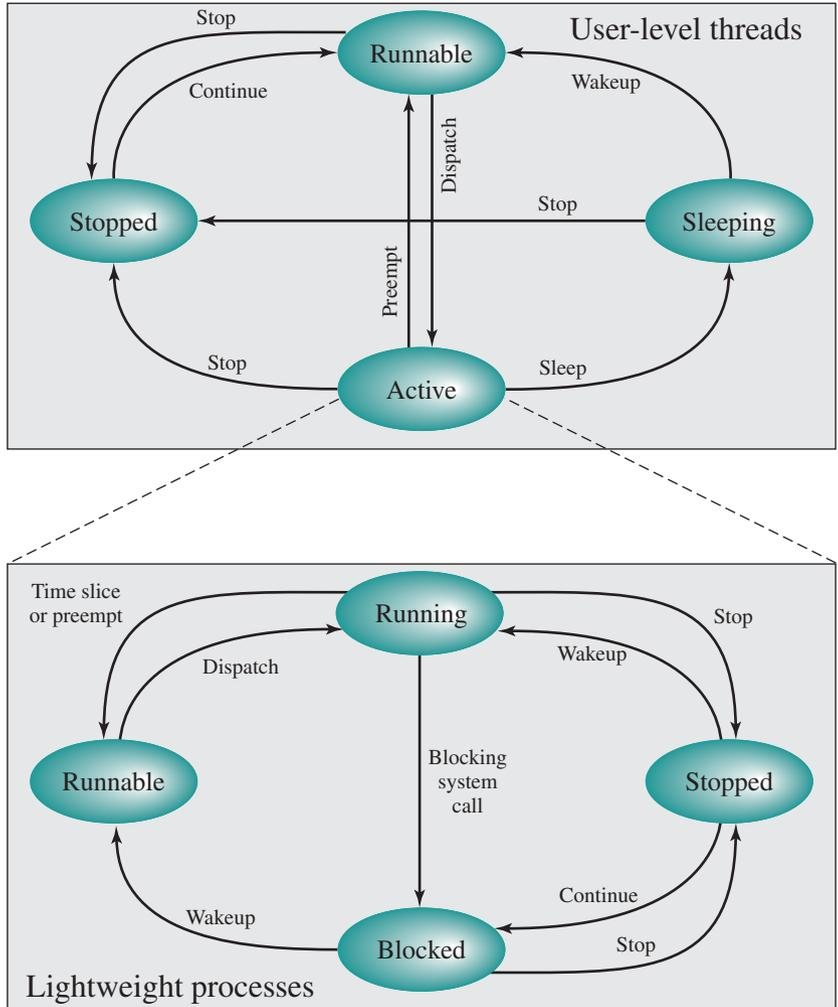
**Figure 4.17** Solaris User-Level Thread and LWP States
