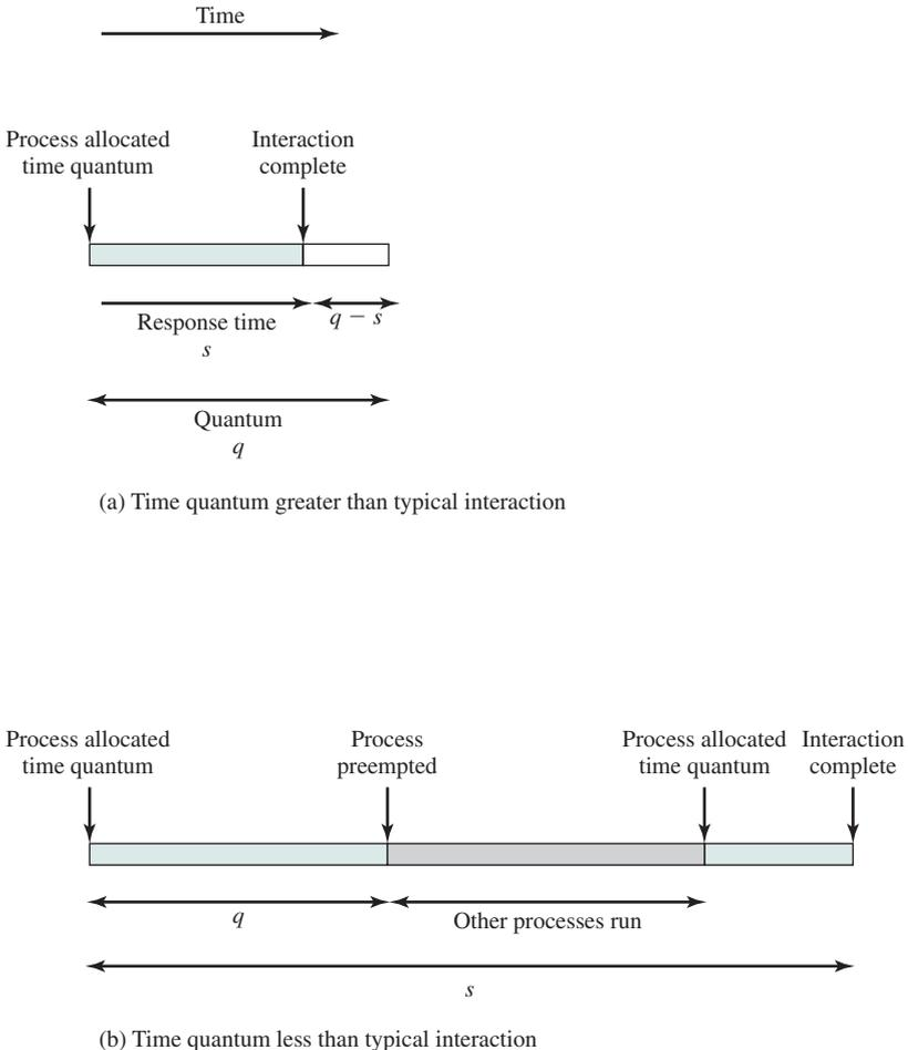
**Figure 9.6** Effect of Size of Preemption Time Quantum
