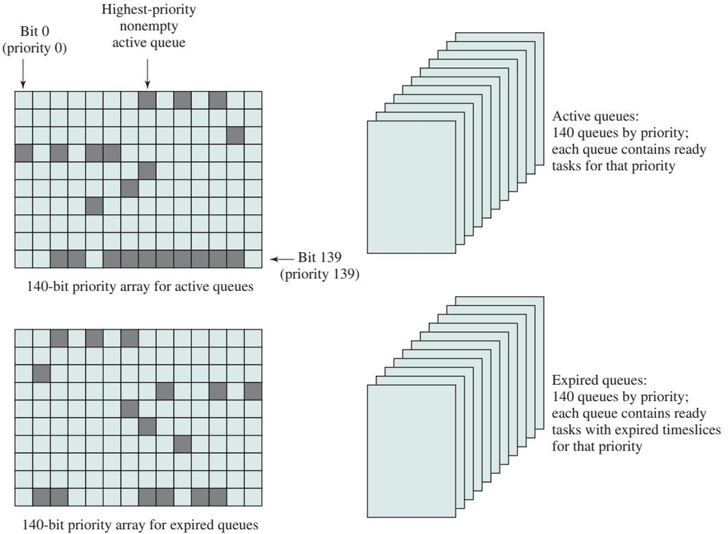
**Figure 10.11 Linux Scheduling Data Structures for Each Processor**
