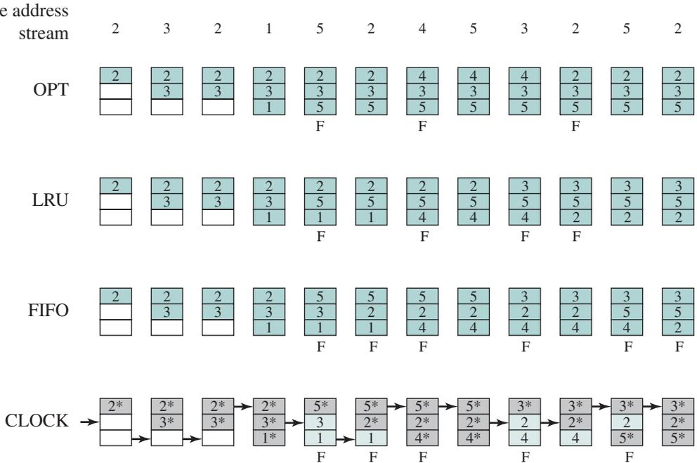
F = page fault occurring after the frame allocation is initially filled
