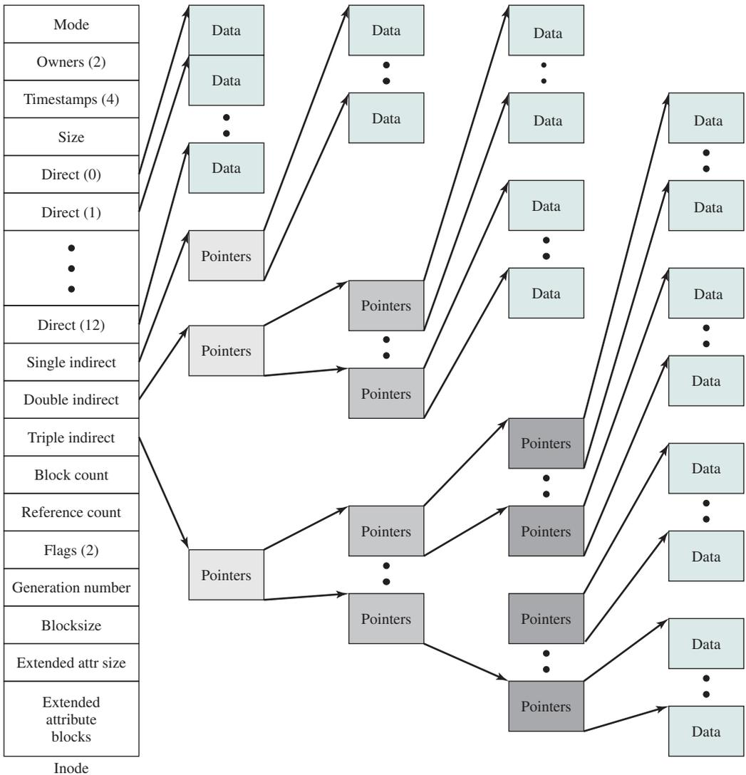
**Figure 12.16** Structure of FreeBSD Inode and File
