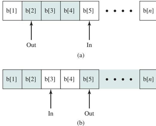
**Figure 5.12** Finite Circular Buffer for the Producer/Consumer Problem
