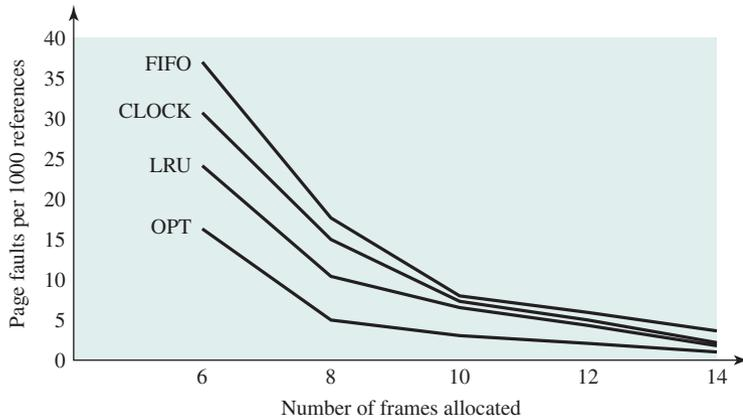
**Figure 8.17** Comparison of Fixed-Allocation, Local Page Replacement Algorithms
