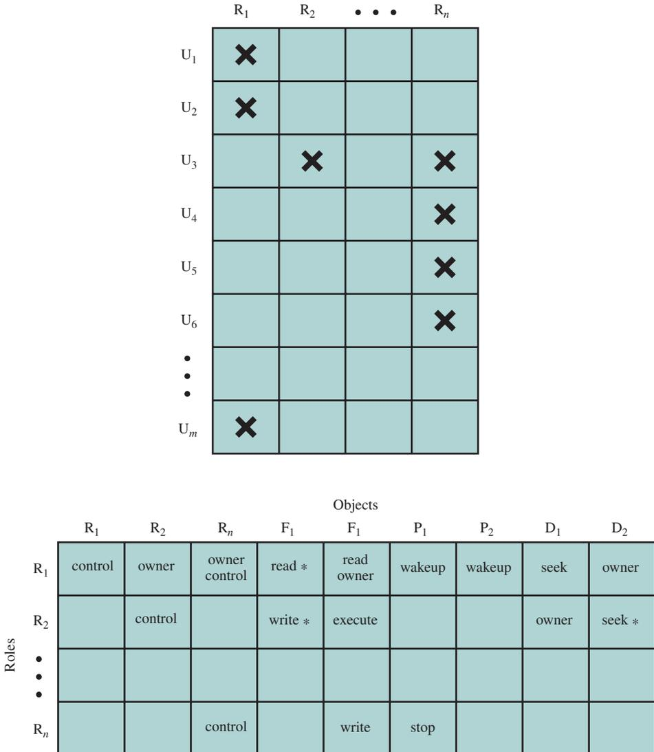
Figure 15.7 Access Control Matrix Representation of RBAC
